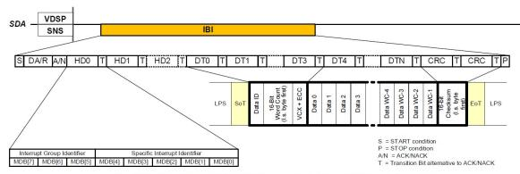
Figure 204 AOSC Smart Transport Mode (STM) Operation for the D-PHY Generic STM Types
