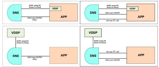
Figure 195 Point-To-Point AOSC Systems with USL Solutions
