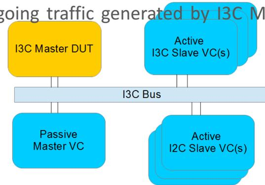
**Active I3C/I<sup>2</sup>C Slave** verification components emulate I3C/I<sup>2</sup>C devices present on the bus. These components should be able to emulate both proper and erroneous behavior, in order to test the ability of DUT to recover from errors in accordance with I3C spec requirements
