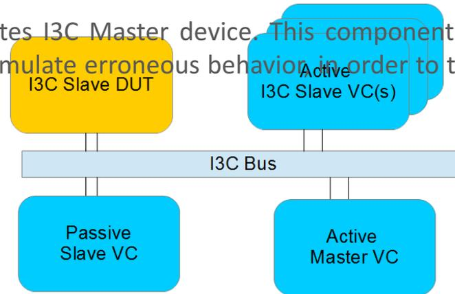
**Active I3C Slave** verification components emulate additional slave devices present on the bus, mostly for testing of arbitration-related aspects
