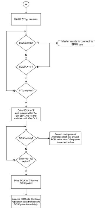
**Figure 32 Detecting Bus Arbitration to Connect to Bus Flow Diagram**
