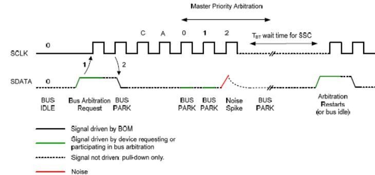
Figure 27 Noise During Priority Slots of the Bus Arbitration
