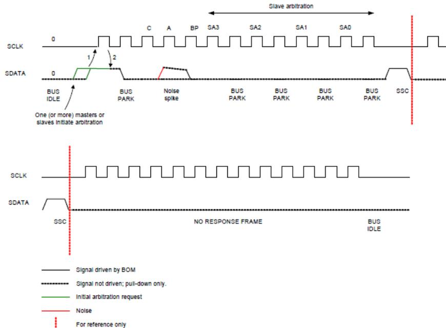
Figure 28 False Slave Arbitration due to Noise
