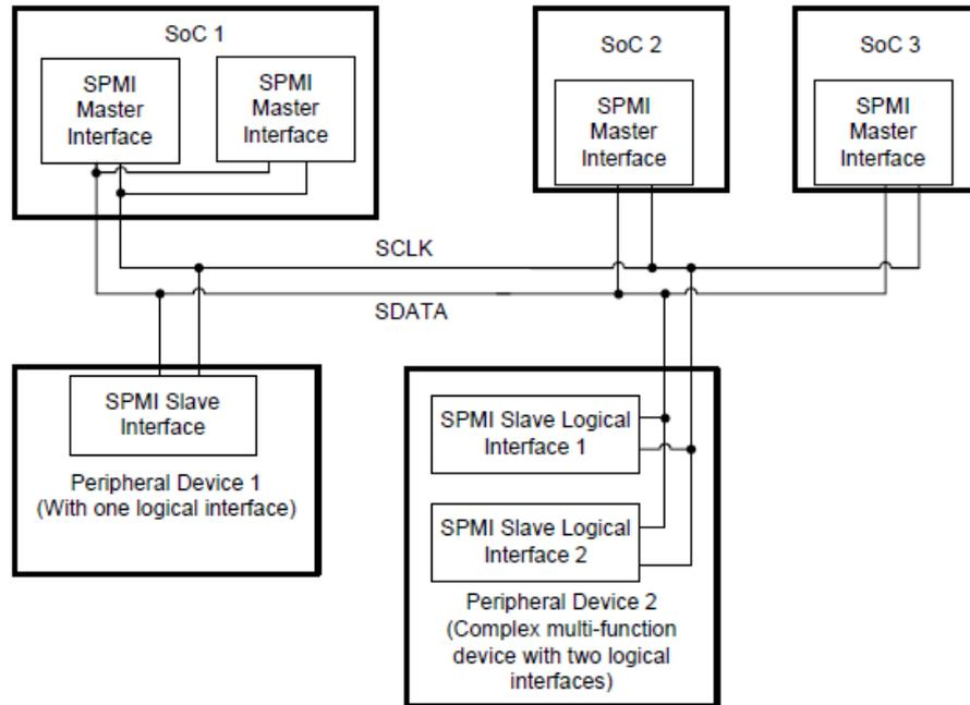
**Figure 1 SPMI System Example**
