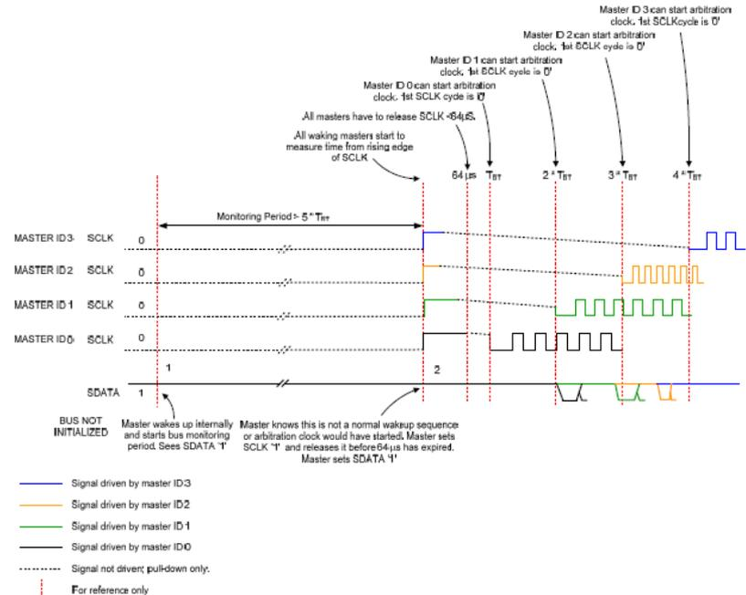
Figure 34 Bus Initialization with Pending Bus Arbitration Request by RCS
