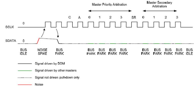
Figure 26 False Bus Request Detection
