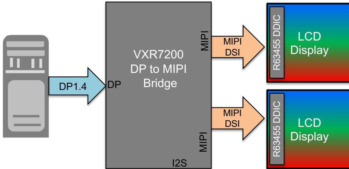
Flexible and Optimized GPU-to-Pixel Video Solution
