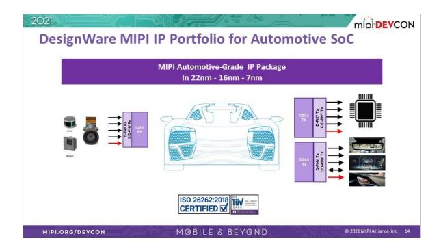
Synopsys' MIPI IP portfolio comprises very comprehensive solutions encompassing controllers from sensors to displays. With the PHY layer of CSI and DSI, the ecosystem includes D-PHY RX to D-PHY TX, from C-PHY/D-PHY RX to C-PHY/D-PHY TX. Our PHY IP is available on 22nm, 16nm, and 7nm processes.
