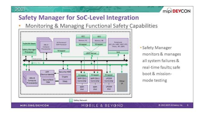
In addition, Safety Manager is often integrated into the design process of automotive-grade SoCs. The purple items in this diagram denote the flow of a traditional IP block, whereas the Safety Manager is shown in green. The objective of the Safety Manager is to monitor and manage all possible system failures, including mission-mode testing. Here, you can see that the entire flow of the MIPI, starting from the wrapper, must conform to Safety Manager requirements.
