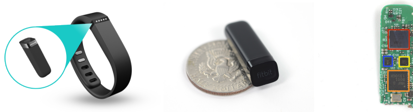
Figure 4: Simple activity tracker Fitbit Flex, product (left), electronic module (middle) and PCB assembly with the accelerometer marked with a yellow square (right). Images from UserLib ( http://www.userlib.com/fitbit-flex-manual-tutorial/ ) and iFixit ( https://www.ifixit.com/Teardown/Fitbit+Flex+Teardown/16050 ).
