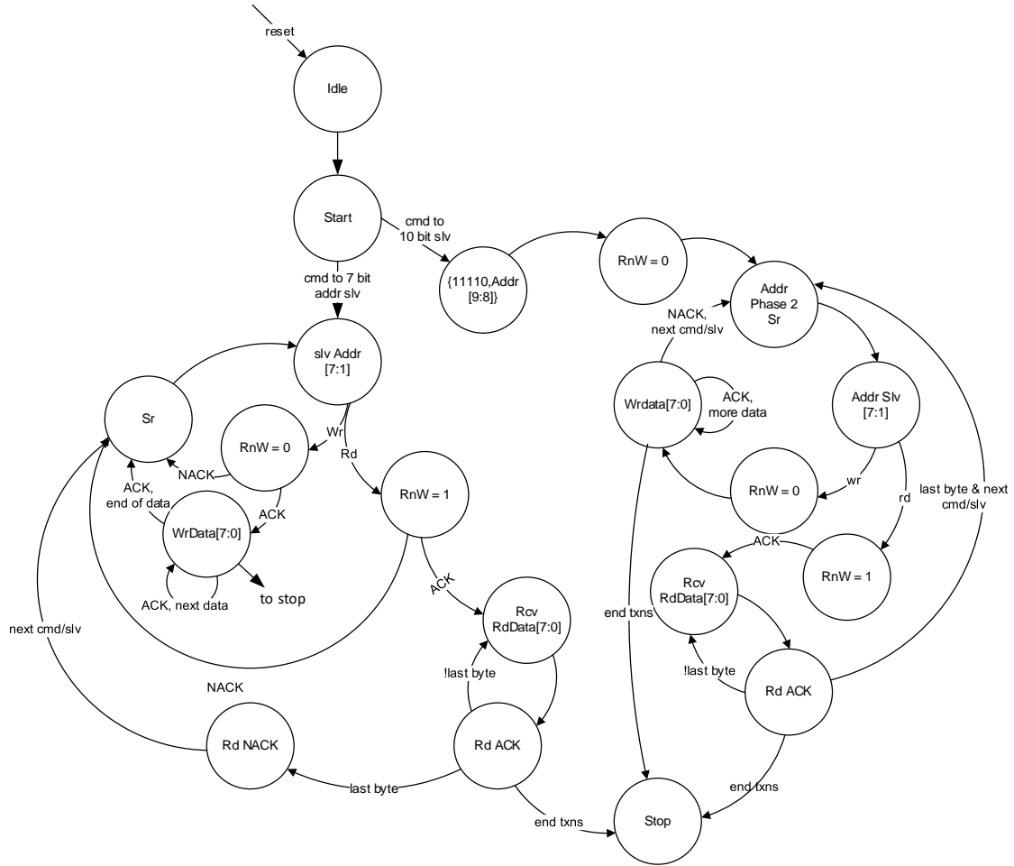
Figure 63 I2C Legacy Master FSM
