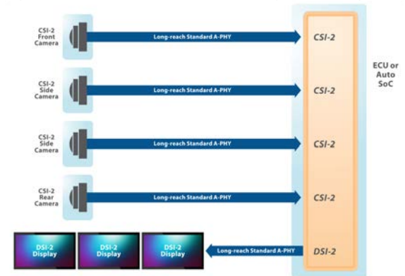
FUTURE INTEGRATED A-PHY IN ENDPOINT CAMERAS (NO BRIDGES: Lower cost, weight, power)
